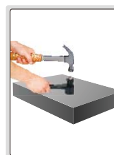
hammer impact to apply test force
